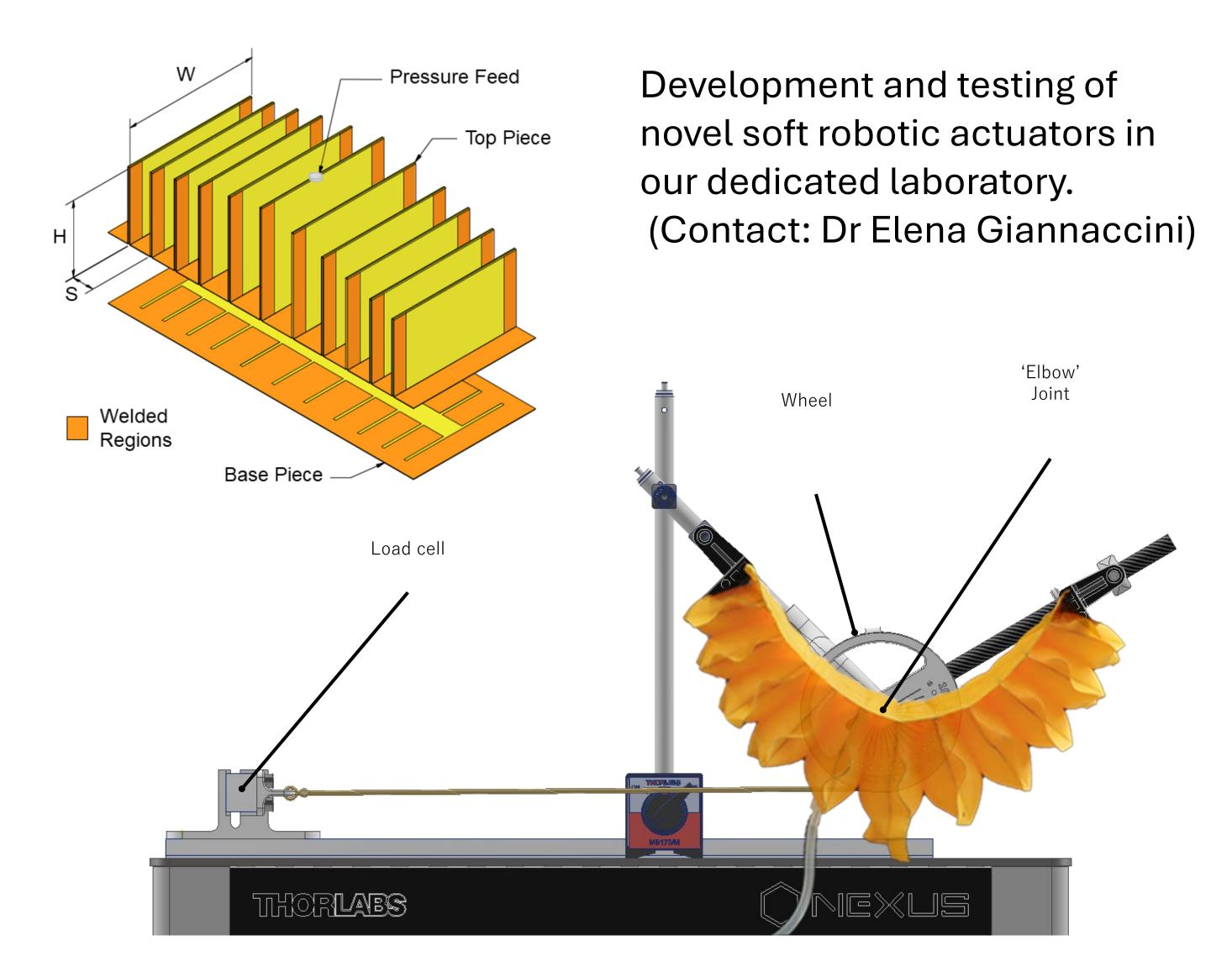
Our work goes from initial design and development, through benchtop testing, to user testing in the biomechanics lab.
