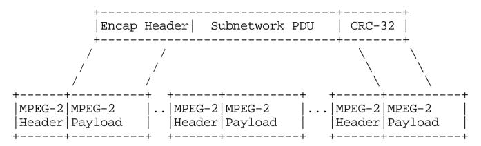
Direct transmission over MPEG-2 TS, use of PUSI IPv4 & IPv6 with support for Header Compression (ROHC) Min MTU 1280 B [RFC 2460]; better 1500 B Eliminate options and reduce per-packet processing
