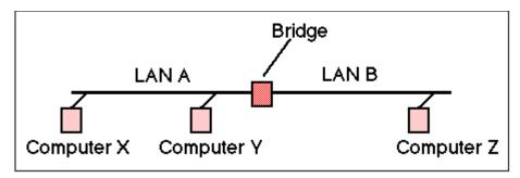
mation to learn which frames need to be forwarded by the bridge. Packets with a source of X and destination of Y are received and discarded, since the computer Y is directly connected to the LAN A, whereas packets from X with a destination of Z are forwarded to network B by the bridge
