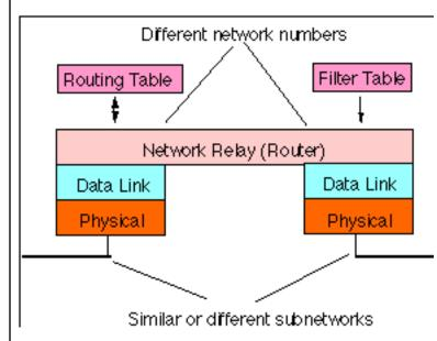
A router is an Intermediate System (IS) which operates at the network layer of the OSI reference model. Routers may be used to connect two or more IP networks, or an IP network to an internet.
