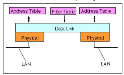
The learned addresses are stored in the corresponding interface address table. Once this table has been setup the bridge examines the destination address of all frames, and forwards them only if the address does not correspond to the source address of a computer on the local subnetwork.
