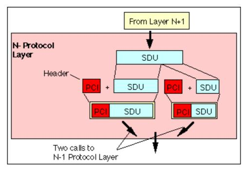
maximum size of the packet payload (Service Dat aUnit (SDU)) which may be supported.
