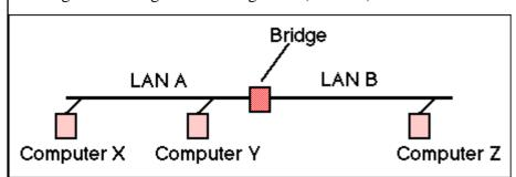
The bridge learns (by observing th feaders of Ethernet frames) whice MAC addresses belong to the computers on each conected subnetwor by observing the source address values which originate on each side of the bridge. This is called "learning' In the figure in the question, the source addresses X,Y are observe to be on network A, while the address of computer Z will be observe to be on network B.
