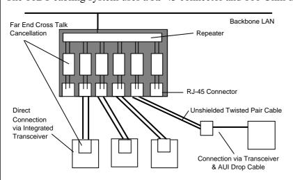
nects the computer directly (i.e. using a point to point link) to a wiring hub which acts as a media repeater. The maximum distance of a 10BT link is 100 m. It is normally used to connect work groups of users, sometimes by wiring an entire floor with outlets to each work area.
