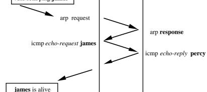
The Address Resolution Protocol (ARP) is used when, percy, a local computer (with Medium Access Control (MAC) address x) wishes to communicate with a remote computer, james, (with mac address y). Redraw the diagram above describing what happens at each stage and provide notes to give a detailed explanation of the operation of ARP. Ensure you specify which addresses are used as the source and destination addresses of each frame. [ 6 marks ]
