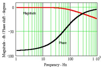
Fig. 2. Frequency and phase response of a  $1^{st}$  order Butterworth filter with cutoff at 600 Hz.
