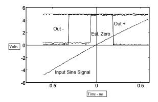
Fig. 4. Oscilloscope capture of the sine wave signal, optoisolator outputs and computed zero crossing.
