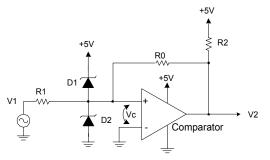
Fig. 5. Resistive feedback hysteresis circuit
