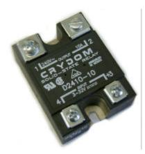
We recommend using standard solid state relays such as the Crydom D2410-10 (Digi-key part # CC1079-ND or RS part # 291-2034 for the D2450-10 {a 50A version}) that will switch 120/240V AC at up to 10A. If using the D2410, connect the DMX receiver outputs to terminals 3 and 4.
