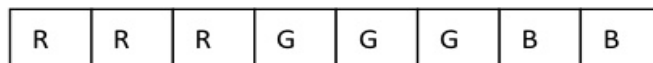
Figure: Mode 1: Format of a Compressed DMX Pixel Control Byte for the Neopixel WS28XX
