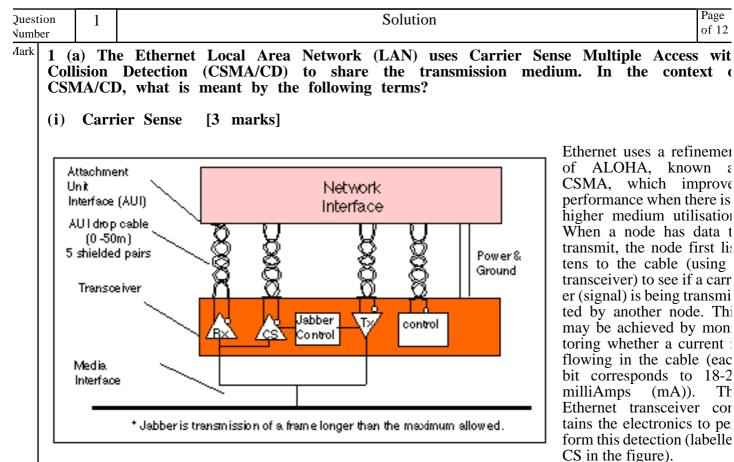
The individual bits are sent by encoding them with a 10 (or 100 MHz for fast Ethernet) clock using Manches ter encoding. Data is only sent when no carrier is observed (i.e. no current present) and the physical medium is therefore idle.
