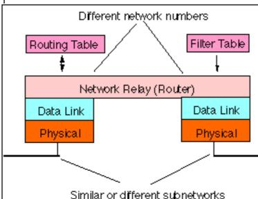
A router is an Intermediate System (IS) whic operates at the network layer of the OSI refer ence model. Routers may be used to connect tw or more IP networks, or an IP network to an in ternet.
