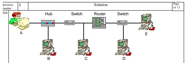
a) The end system A uses the Transmission Control Protocol (TCP) to send a packet to end system D with a payload of 100B, sketch the Ethernet frame that is sent. Ensure you show the addresses at both the MAC and IP layers. [6 marks]
