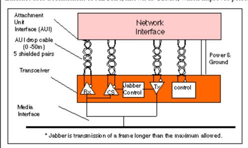
medium utilisation. When a node has data to transmit, the node first listens to the cable (using a transceiver) to see if a carrier (signal) is being transmitted by another node. This may be achieved by monitoring whether a current is flowing in the cable (each bit corresponds to 18-20 milliAmps (mA)). The Ethernet transceiver contains the electronics to perform this detection (labelled CS in the figure).
